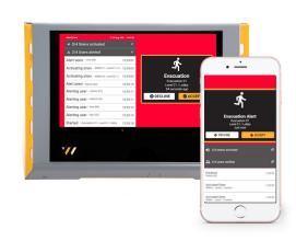
1) An evacuation alert is triggered by the smartphone app (nominated user) or from the TCU 2) Evacuation signal is sent to nominated personnel for optional approval OR automatically pushed out to the rest of the system
